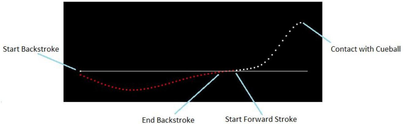
Note that in this sample shot the velocity is negative (moving backward) during the back stroke, motionless during the pause between the end of the backstroke and start of the forward stroke, and positive (moving forward) after the start of the forward stroke. The velocity is increasing up to contact with the cue ball indicating acceleration 'through the cue ball'.
