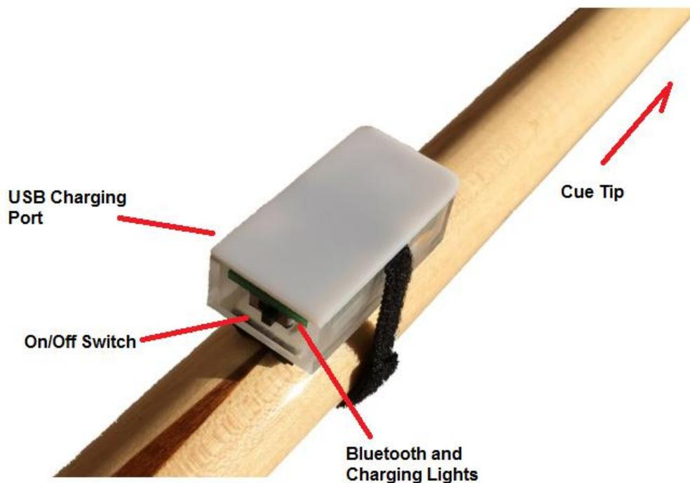
Slide the On/Off switch to the left to power on your unit, to the right to turn it off.
