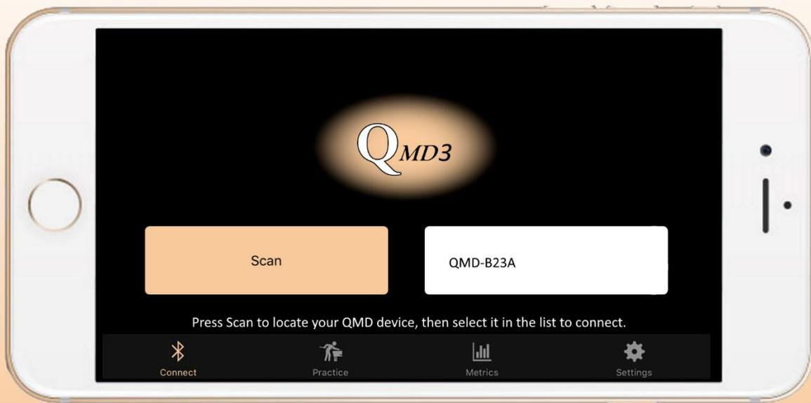
Your QMD3 unit should be mounted on your cue stick, turned on and its blue light blinking for a connection to be started. First, click the **Scan button** to locate your device, it will be shown in the white list box to the right of the Scan button. To complete the connection press your device in the list. In a moment the connection will be completed and the software will automatically switch to the Practice screen.
